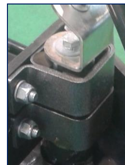
VIB AR-T mounted with VIB clamp SR
